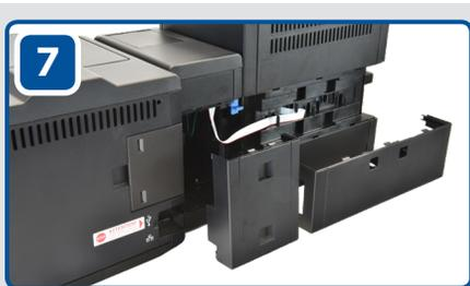
7 Replace the dual side module and lamination module access covers.
