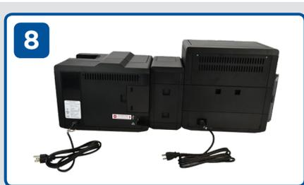
8 Connect the power cords to the printer and the lamination module.
