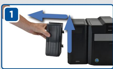
1 Remove the output bin from the dual side module (if attached).
