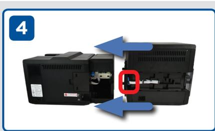
4 Move the blue lever on the lamination module down. Align the posts and slide the lamination module into place. Move the blue lever up to lock.
