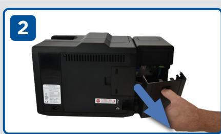
2 Remove the access cover from the dual side module.
