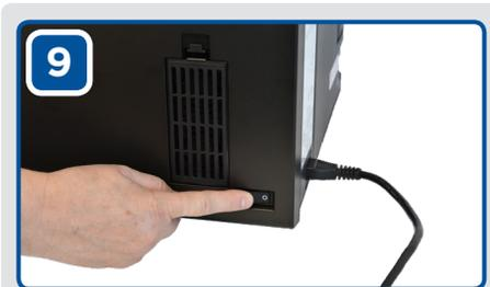
9 Connect the USB/Ethernet cables to the printer (as required) and switch on the printer.
