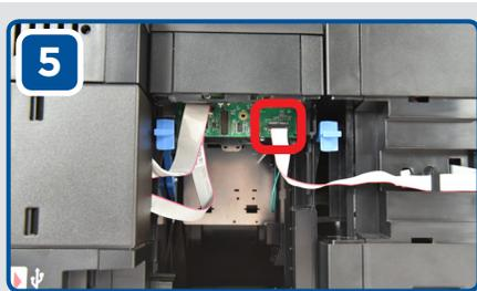
5 Connect the lamination cable to the connector on the dual side module.
